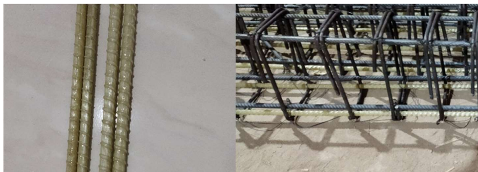
FIGURE 1. Produced GFRP and Steel Bars
